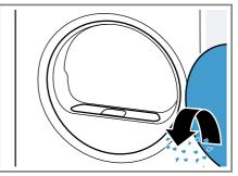
3. Remove the two-part fluff filter.
