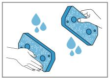
You can remove heavy soiling carefully using a vacuum cleaner. Do not clean the filter mat using cleaning products.
