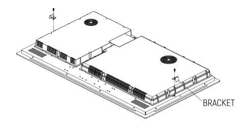
After installation adjust the bracket position to suit for different table top thickness.
