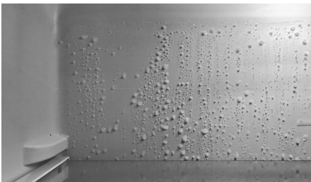
Rear wall showing Ice Droplets during Cooling Phase.
