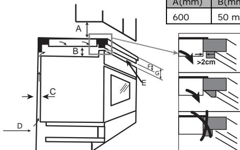
Note: There must be a 560x5mm opening in the front (position E) to dissipate the air.
