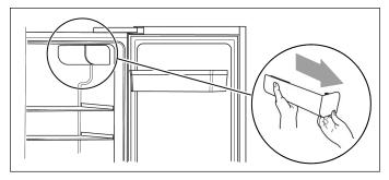
Open the refrigerator door to its maximum angle and remove the water filter cap by pulling it out slowly.
