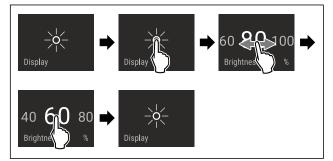
Fig. 67 Example illustration: Switch from 80 % to 60 %.
