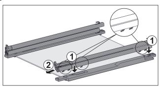
Fig. 154 Glass shelf with rails and retaining parts Install rail with damping mechanism:
