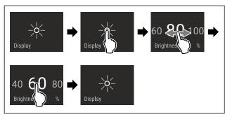
Fig. 62 Example illustration: Switch from 80 % to 60 %.
