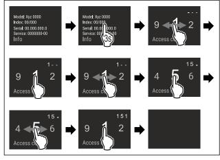
Fig. 5 Example illustration, access with numerical code **151**
