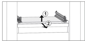
Fig. 102 Example illustration of glass shelf
