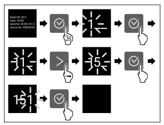
Fig. 4 Example illustration, access with numerical code 151
