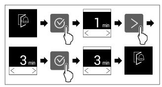
Fig. 46 Example illustration: Change door alarm from 1 minute to 3 minutes.
