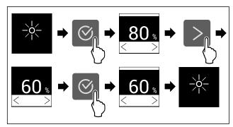
Fig. 44 Example illustration: Switch from 80 % to 60 %.
