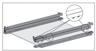
Fig. 110 Glass shelf with rails and retaining parts
