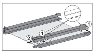
Fig. 114 Glass shelf with rails and retaining parts Install rail with damping mechanism:
