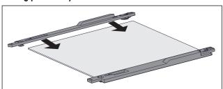
Fig. 112 Glass shelf with retaining part
