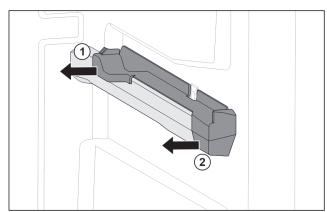
Fig. 107 Attachment on the right moulded rib
