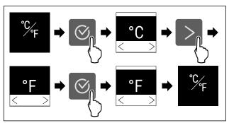
Fig. 20 Example illustration: Switch from degrees Celsius to degrees Fahrenheit.
