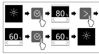
Fig. 53 Example illustration: Switch from 80 % to 60 %.
