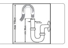
**IMPORTANT:** Items will not wash properly if the drain hose is longer than 4m.
