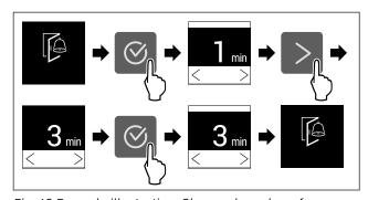
Fig. 42 Example illustration: Change door alarm from 1 minute to 3 minutes.
