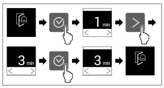
Fig. 50 Example illustration: Change door alarm from 1 minute to 3 minutes.
